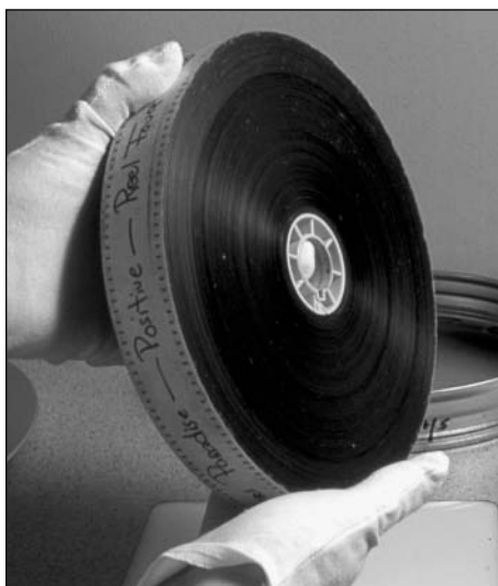
Brace the core with your hand to prevent it from popping out.
