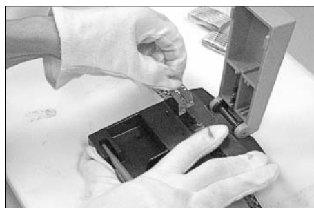
Making a splice using presstape.
